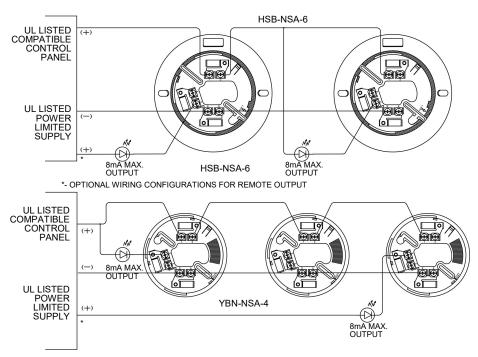
NOTE: Fire alarm control panel compatibility is required for DCP products. DCP communications protocol allows system components (DCP sensors AIE-EA, ALG-V, ACA-V, ACC-V, ALK-V, ALN-V, ATJ-EA and ATG-EA, bases and modules) to be used concurrently on a system's SLC (Signaling Line Circuit).
