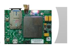
The CLM412/422 is an LTE, category 1 cellular add-on that allows the *FORCE Series* intruder alarm systems<sup>1</sup>, to communicate over a cellular network. The add-on is mounted on the control panel's circuit board and is supplied with an antenna.
