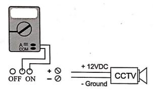
To determine the current(A)draw of a camera remove the jumper link, set your meter to- A/ Amps DC, and with the camera connected measure the current across the ON and COMMON terminals.
